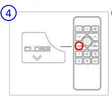
Short press the CLOSE button on the remote to set the fully-closed limit.
