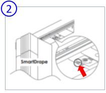
Press the button 3 times fast to the pairing mode. Blue light flashes for 1 min.
