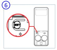
Press the SET button on the remote for 3 seconds to leave the SET mode. Remote light out.
