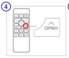
Short press the OPEN button on the remote to set the fully- opened limit.
