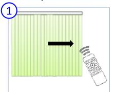
Expand all fabric vanes and rotate the vanes to fully-closed position (privacy).
