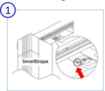
Make sure the motor is powered on. Press the button 3 times fast to start the pairing mode. Blue light flashes for 1 min.
