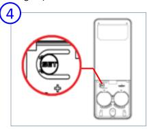
Short press the RESET button on the remote to set the special limit.
