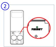
Long press RESET button on the remote. All group numbers on the remote light on and flash fast.
