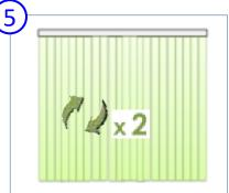
The fabric vanes rotate twice if the unpairing is done. The light goes out.
