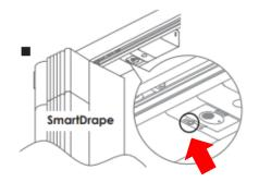
**Power on**: Press the button for 3 seconds. Blue light flashes 4 times, and buzzer sounds twice.
