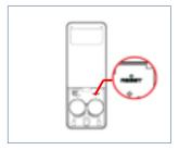
Long press RESET button on the remote. All group numbers on the remote light on and flash fast.
