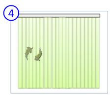
The fabric vanes rotate if the pairing is done. The light on the motor goes out.
