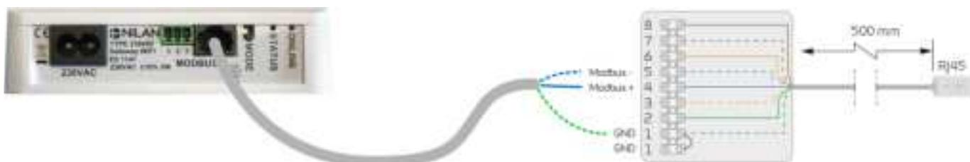
The illustration shows the process when using a type A LAN cable
