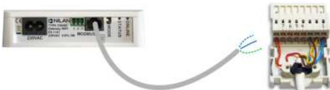
The illustration shows the process when using a type A LAN cable
