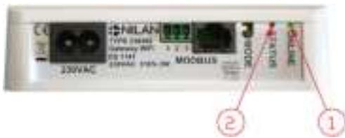
1. The ONLINE indicator makes it possible for you to check the connections by using the following code:
