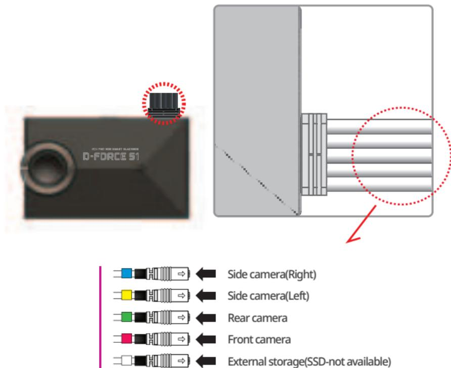
※ Side cameras are recorded with the function of mirrored mode.
