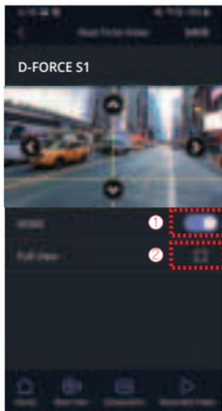
① To improve the ADAS recognition rate, it is recommended to adjust the dash camera position by matching the end of the vehicle bonnet line on condition that "the lane correction button" is turned on in the real time screen.
