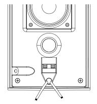
③ Run the speaker cable through the tube positioned at the rear of the cabinet to the terminal at the front baffle.
