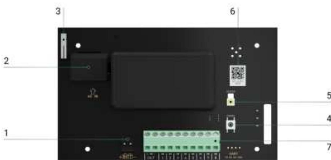
1. Terminals for connecting a 12 V<sub>DC</sub> backup battery.
