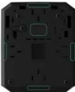
4. Fasten the casing to a vertical surface at the chosen installation location using the bundled screws. When attaching, use all the fixation points on the casing. One of them, in the perforated part of the mount above the tamper, is needed to trigger the tamper on the back of the board in case of an attempt to tear the casing off the surface.
