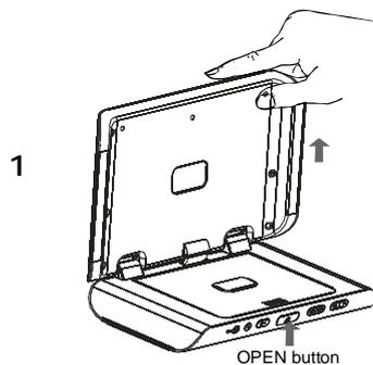
**1** Open TFT cover first, then press OPEN button to open the disc cover.
