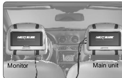
1. Connect the two players with AVP cable first, and then plug the car power cable to DC IN socket of the main unit.
