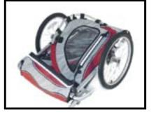
The trailer can be folded with or with out the wheels on. If the wheels are removed they can be stored inside the trailer when not in use.
