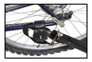
Unhook the safety strap from the loop. Loosen the knob to open the hitch.
