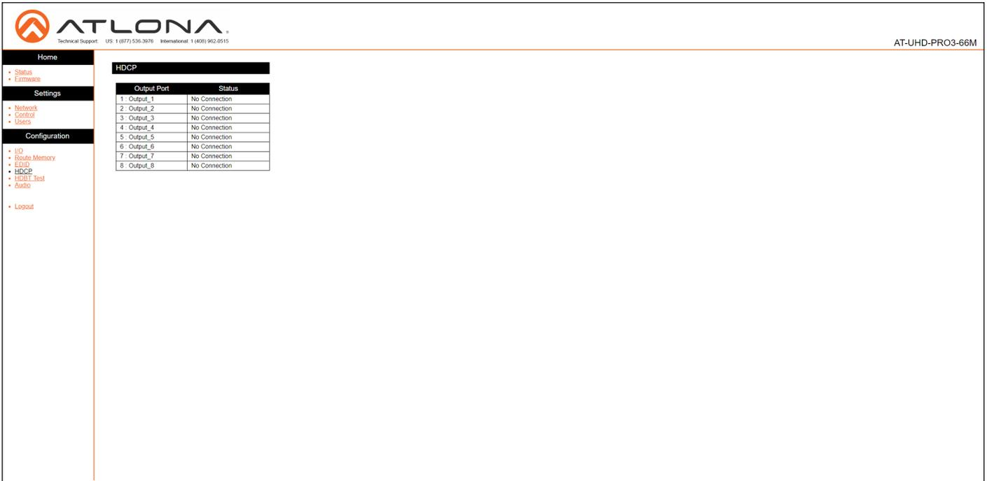
The screenshot shows the ATLONA web GUI interface. At the top left is the ATLONA logo and contact information. The top right corner displays the model number AT-UHD-PRO3-66M. A navigation menu on the left side includes sections for Home, Settings, and Configuration. The main content area is titled 'HDCP' and contains a table with two columns: 'Output Port' and 'Status'. All eight output ports listed in the table show a status of 'No Connection'.
