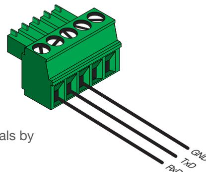
10. Locate the included 3-pin captive screw block and open each of the terminals by turning the screws counter-clockwise, using a small regular screwdriver.
