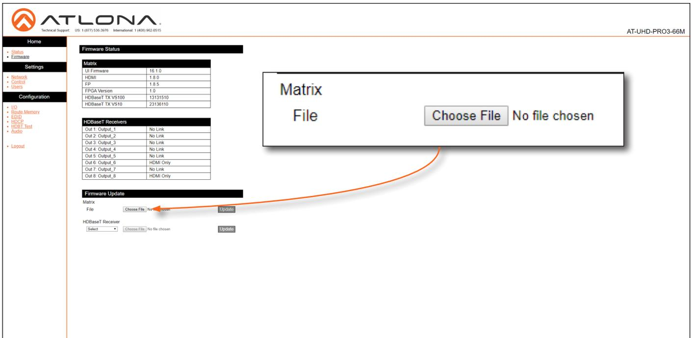
The screenshot shows the ATLONA web GUI interface. On the left is a navigation menu with 'Home', 'Status', 'Firmware', 'Settings', 'Configuration', and 'Logout'. The main content area is divided into three sections: 'Firmware Status', 'HDBaseT Receivers', and 'Firmware Update'. The 'Firmware Update' section contains a 'Matrix File' label, a 'Choose File' button, and an 'Update' button. A callout box with the text 'Matrix File' and 'Choose File No file chosen' points to the 'Choose File' button.
