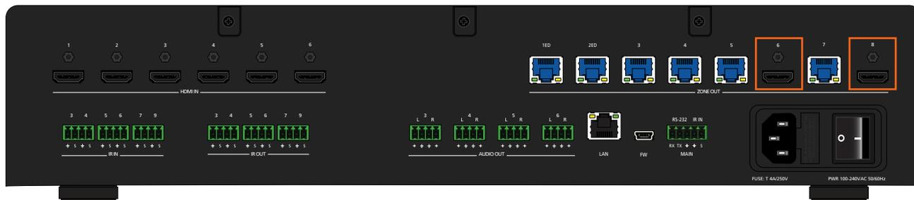
These two HDMI ports are used to mirror (duplicate) an HDBaseT output signal and to either or both HDMI output ports. By default, mirroring is enabled on these two ports. However, mirroring can be disabled. When mirroring is disabled, any of the six HDMI inputs can be routed to these HDMI outputs, transforming this product into an 6 x 8 matrix switcher. The default mirror settings are listed below
