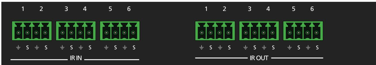
3. Insert the GND and Signal leads into correct terminal, as shown, and tighten the screws to secure each wire. Do not overtighten.
